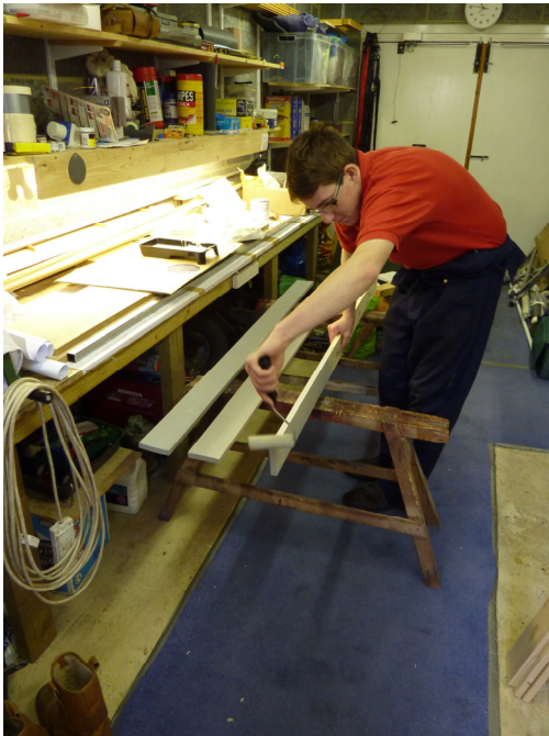
Left – Early January 2011 and Alistair applies primer to the planks that will eventually form the sides and ends.
