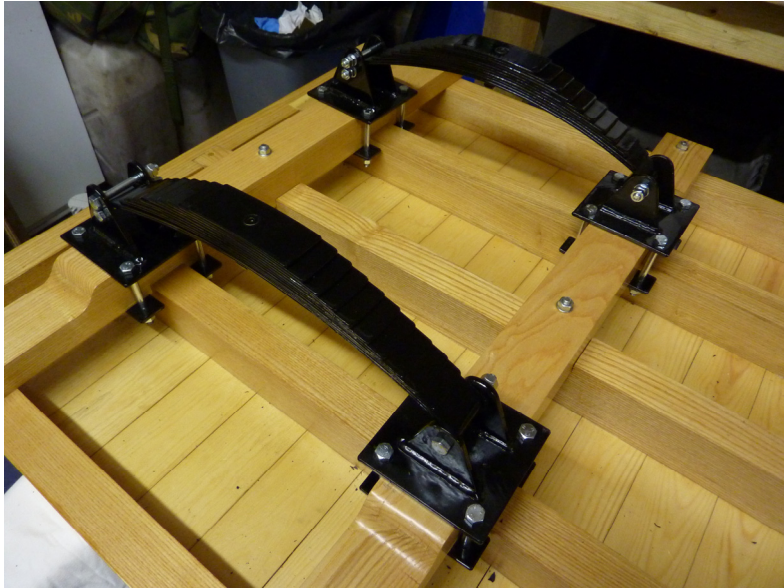
Left - Early March 2011 and the springs are fitted to the hangers. What we have now is basically a kit of parts to assemble, the really hard work is over.
