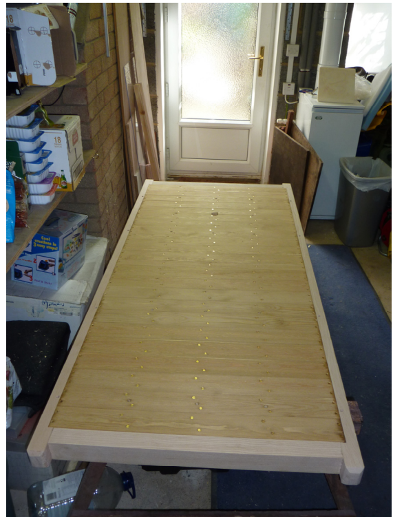
Above – By the 10 th May the frame was coming together and by August the bed, including the planking, had been completed. The latter held in place with 230off 20mm x 8 countersunk brass screws all screwed in by hand and finished with their slots in line with the grain. 3 coats of yacht varnish followed. It was a very impressed dad that upon assembly of the four external members, noted that the diagonals were within a millimetre of each other – some pretty accurate mortice and tenon joints there then.
