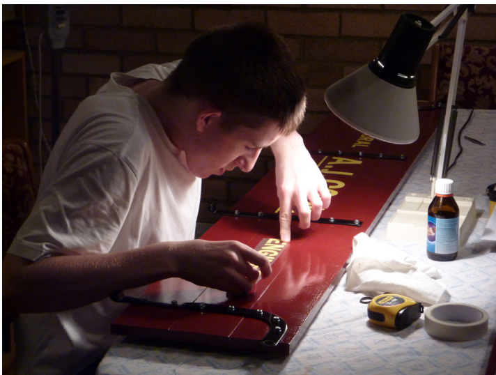
Left - You can almost hear the concentration as the vinyl 'signwriting' is applied. Each section comprising two sets of letters, cream on black shadowing, makes the task even more stressful as the backing adhesive only has to touch another surface and it 'bites'.
