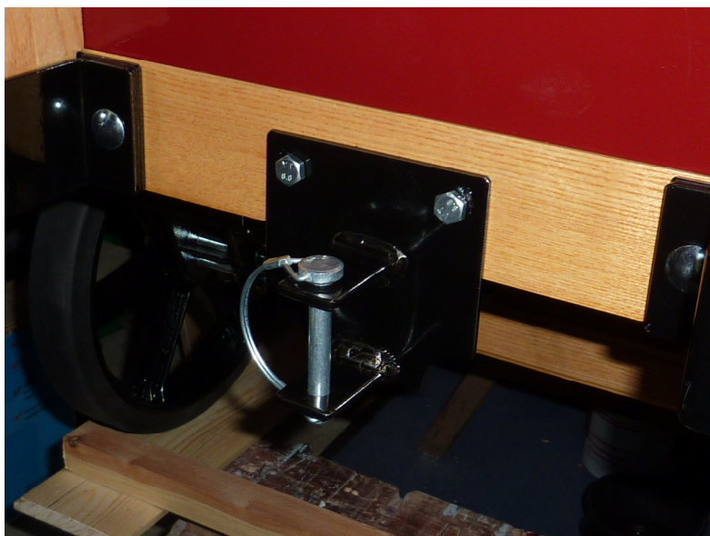
Left - Close up of the towing hitch, necessary for the bowser which is the next project - the 80ltr. tank is made, it just needs a chassis, springs, axle and wheels!
