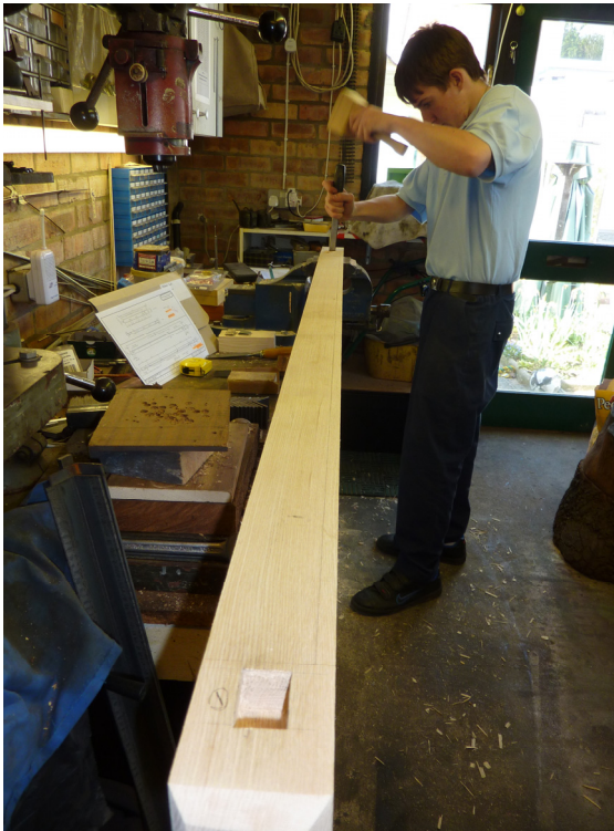
Above – It was the 3 rd of May 2010 before the drawings were sufficiently advanced for Alistair to make a start. Aware of the enormity of the task ahead, his dad had procured the English Ash in planed lengths of 44 x 66 mm section, both to ease the workload and speed the progress.
