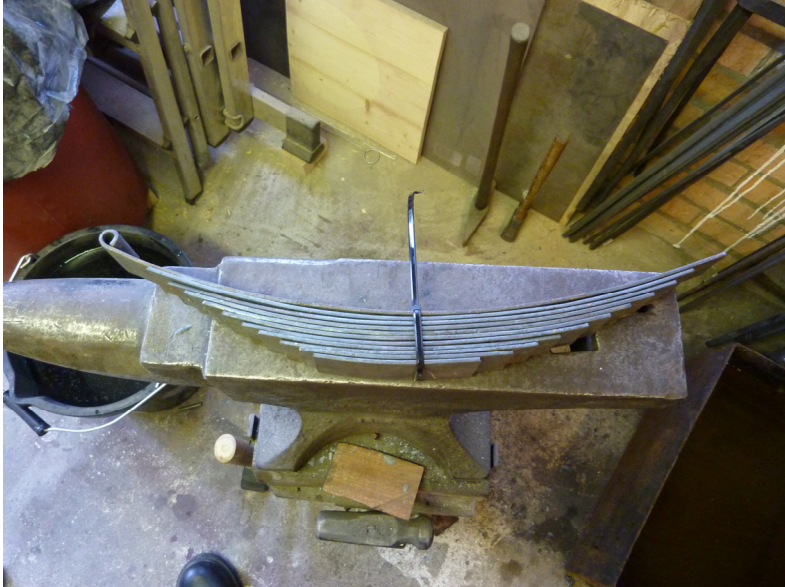
Left – A full set of 11 leaves, all to be cleaned, drilled, bolted and painted.
