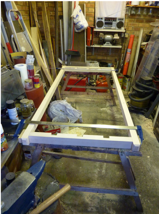
Above – By the 10 th May the frame was coming together and by August the bed, including the planking, had been completed. The latter held in place with 230off 20mm x 8 countersunk brass screws all screwed in by hand and finished with their slots in line with the grain. 3 coats of yacht varnish followed. It was a very impressed dad that upon assembly of the four external members, noted that the diagonals were within a millimetre of each other – some pretty accurate mortice and tenon joints there then.
