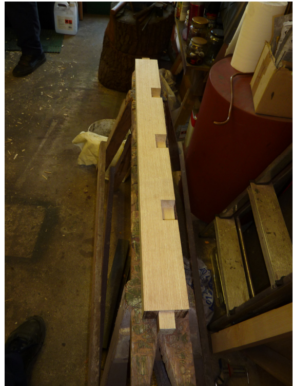
Above – It was the 3 rd of May 2010 before the drawings were sufficiently advanced for Alistair to make a start. Aware of the enormity of the task ahead, his dad had procured the English Ash in planed lengths of 44 x 66 mm section, both to ease the workload and speed the progress.
