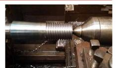
At one end is a tapered section and a thread for attaching the piston. I had to take great care to match the taper inside the piston, which ensured a tight fit. The thread is cut with a process called screw-cutting where a special tool is
